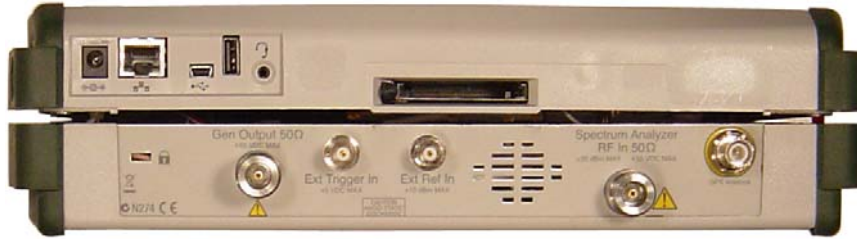
Figure 3-6. MS272xB Case Halves Partially Separated
